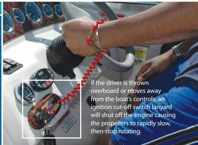
If the driver is thrown overboard or moves away from the boat's controls, an ignition cut-off switch lanyard will shut off the engine causing the propellers to rapidly slow, then stop rotating.
